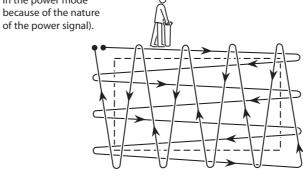
Trace the buried conductor keeping the C.A.T<sup>3</sup> vertical and moving it steadily from side to side. Follow the line of the buried conductor marking it with chalk or paint across the area to be excavated.
