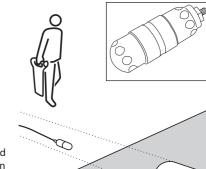
Smaller ghost signals appear before and behind the main signal position. Locate all three peaks to be sure the largest middle one is identified as the Mouse position.
