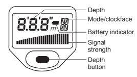
The main features of the C.A.T<sup>3</sup>V and C.A.T<sup>3</sup>+ are the same as the C.A.T<sup>3</sup> but the addition of a liquid crystal display brings further features.
