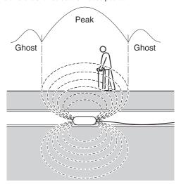
Rotating the C.A.T<sup>3</sup> about it's axis to obtain the largest signal puts the blade of the C.A.T<sup>3</sup> in line with the Mouse and is a good way of identifying the direction of the duct or pipe.
